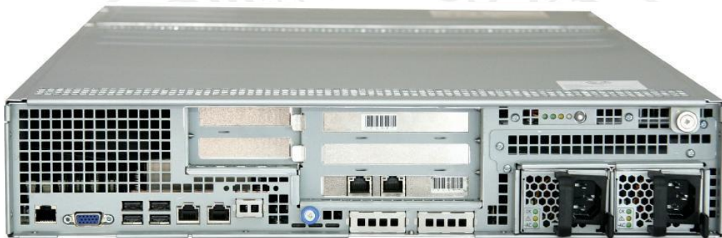
PICTURE 2: Intel SR2612UR server - back panel
