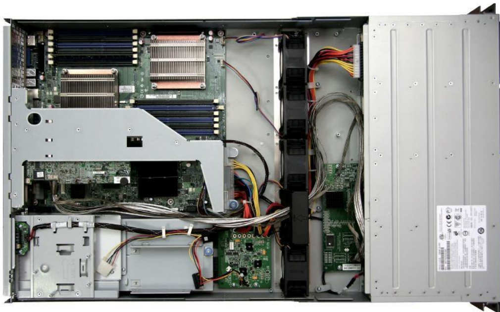
PICTURE 3: Intel SR2612UR server - inside
