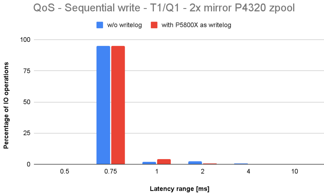
Fig. 21. Latency distribution for a sequential write test, done on a 2x 2-way mirror SSD zpool (T1/Q1), with and without writelog.
