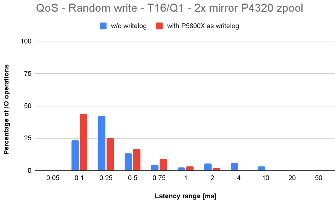
Fig. 19. Latency distribution for a random write test, done on a 2x 2-way mirror SSD zpool (T16/Q1), with and without writelog.
