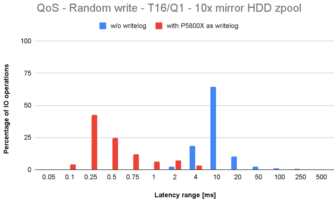
Fig. 7. Latency distribution for a random write test, done on a 10x mirror HDD zpool (T16/Q1), with and without writelog.
