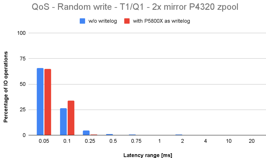
Fig. 18. Latency distribution for a random write test, done on a 2x 2-way mirror SSD zpool (T1/Q1), with and without writelog.
